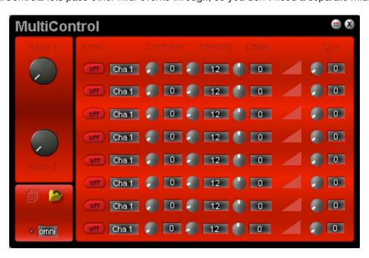
Knob 1 + 2: Main knobs, which control the assigned control output
